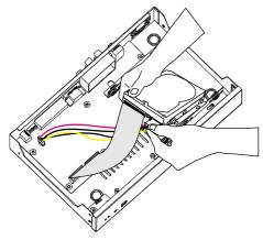
6. Secure the hard disk inside the unit then replace unit cover
